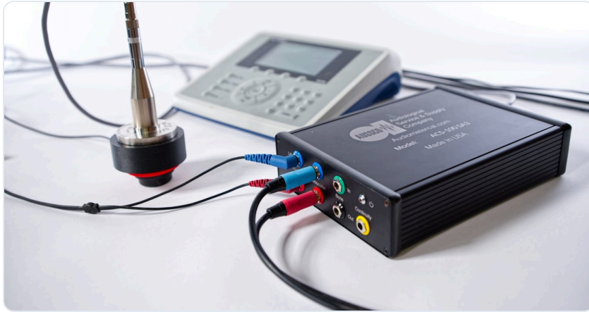
ACS-100 SA3 connected to an audiometer; microphone mounted on a coupler.
